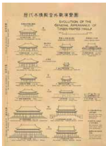
Evolution of the General Appearance of Timber-framed Halls by Liang Sicheng in the 1930s.
