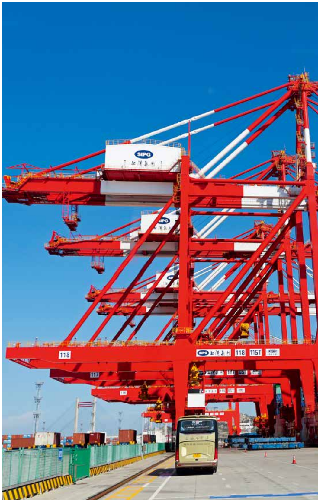
The fourth phase of Shanghai's Yangshan Deep-Water Port is the world's largest unmanned container terminal, with the highest degree of automation. by Qiao Zhenqi
