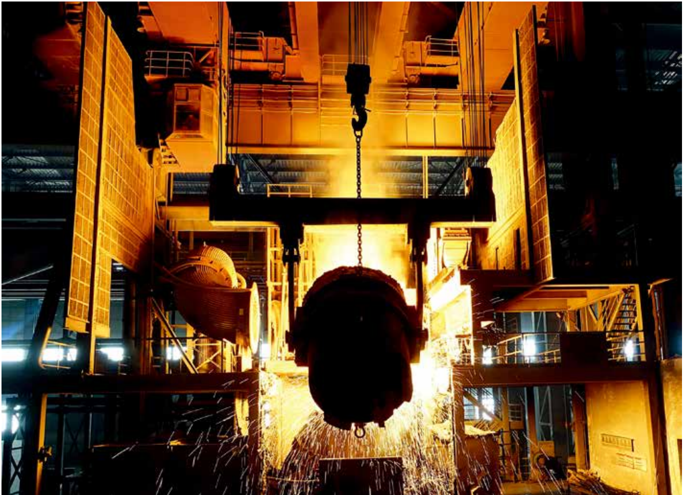
February 12, 2018: Workers from Dalian Special Steel Products Co., Ltd. pour molten steel into an AOD furnace. VCG
